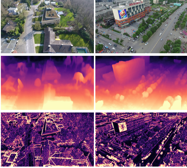
Fig. 2. Illustration of the uncertainty maps. The 1st row shows the input images, the 2nd row shows the predicted depth maps, and the last row shows the estimated uncertainty maps, which mostly highlight rapidly-changing pixel regions including vehicles and building edges.
